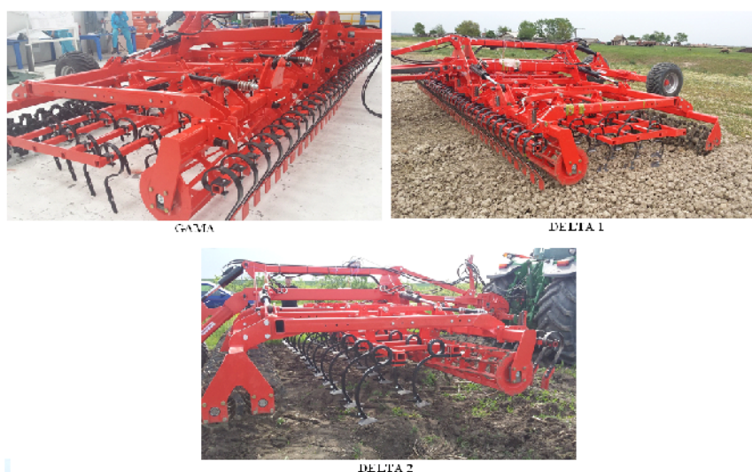
Figure 3. The prototype vibro-combinator SANDOKAN 2 equipped with the three types of active elements (GAMMA, DELTA1, DELTA2) [21,22]
